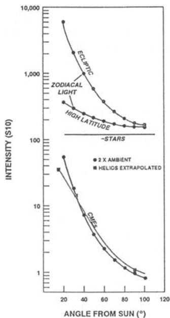
**Figure 1.** The brightness of various signals that will be observed by the imager versus elongation at 1 AU.
