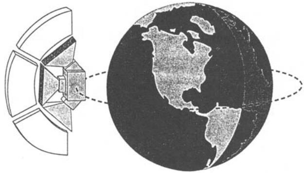
**Figure 2.** SMEI in a typical equatorial orbit. The spacecraft orbit is circular at 800 km above the surface of the Earth.
