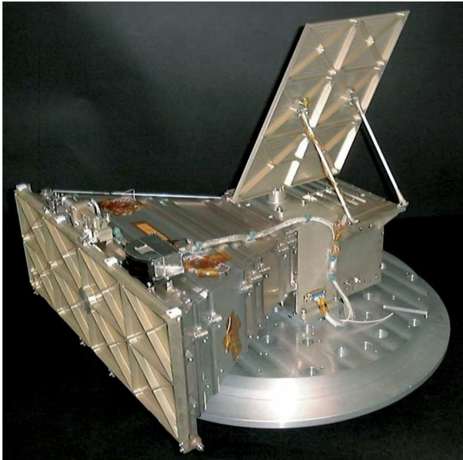
Figure 2. One of the three SMEI camera units, shown mounted to an interface plate which was used in vibration qualification.
