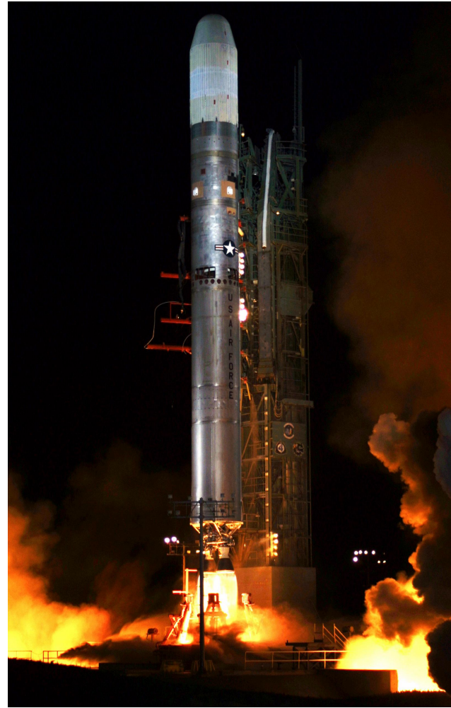
Figure 1 (a) Coriolis spacecraft with the Solar Mass Ejection Imager (SMEI) instrument on board prior to launch. The three instrument camera baffles (circled). (b) Titan II launch of the Coriolis spacecraft on 6 January 2003 with on board SMEI and WindSat.
