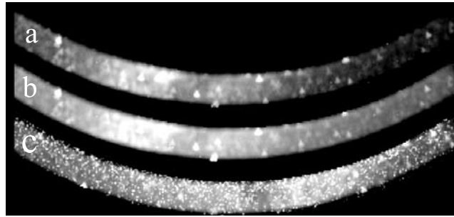
Figure 3. Examples of the effect of aurora and charged-particle strikes on raw SMEI data frames. All are from the middle camera. (a) A normal frame, taken 7 November 2004, 1554 UT, during a north polar cap passage. (b) The same region of the sky two orbits later, showing uniform elevated levels due to presence of aurora. (c) A frame taken three minutes following the second, showing the granular effect of charged particle strikes on the CCD.
