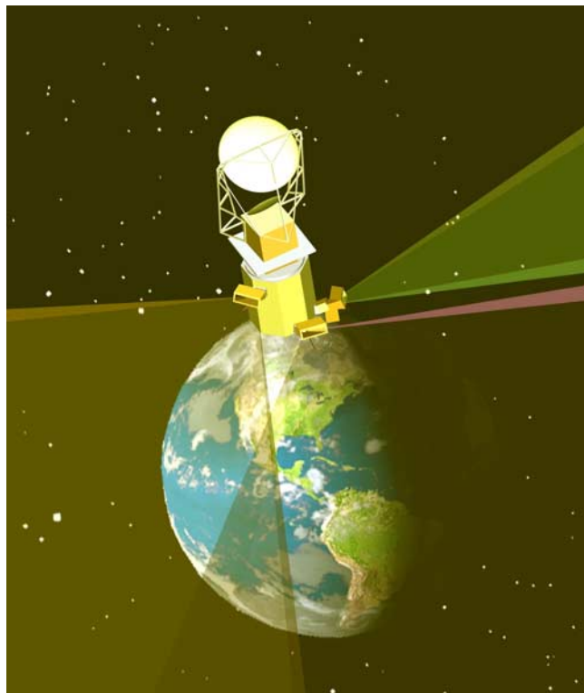
Figure 1. SMEI is depicted on the Coriolis spacecraft in its terminator polar orbit at 840 km with an orbital inclination of 98^\circ . SMEI looks away from the Earth at 30^\circ above the local horizontal to avoid sunlight reflected from the Earth and from the Windsat radiometer antenna situated at the top of the Coriolis spacecraft. The fields of view of the three cameras (each shown as shaded wedges extending from the satellite in this artist's impression) together cover nearly 180^\circ of sky and, as the instrument orbits Earth, sweep out nearly the whole sky around it.
