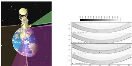
**Figure 1:** (left) Coriolis in its dawn-dusk terminator orbit. The fans indicate the fields of view of the three SMEI cameras. (right) 4-sec exposures from camera 3 of the same section of sky one year apart (2003-2006) after correction for pedestal and dark current. Stars appear as fish-shaped structures on the inner edge, and move across the 3° FOV in about a minute.
