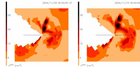
**Figure 4.** 3D SMEI tomographic reconstruction in electron density for these same heliospheric structures at 00:00 UT on 9 (left) and 10 (right) November 2004 (adapted from Bisi *et al.*, 2007). As in Figure 3, an r<sup>2</sup> radial density fall-off has been removed from the analysis.
