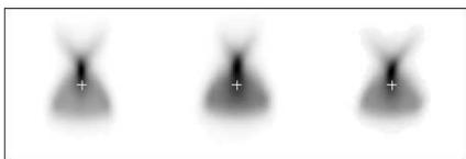
**Figure 1: The full-sky PSF for cameras 1, 2 and 3 (left to right) in equirectangular projection. The crosses indicate the centroid. This PSF was determined empirically using stars with no close neighbours. For each camera a  $2^\circ$  square is shown. This "standard star" can be viewed as a star with its centroid at the vernal equinox with  $\theta=0$  (see below).**
