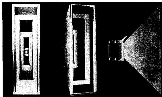
Fig. 4. Photograph of the test baffle constructed at the University of California at San Diego for the proposed WIND imager.
