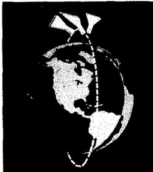
Fig. 3. Orbit of a typical DMSP satellite (9am - 9pm). The spacecraft orbit is circular at 800km above the surface of the Earth and maintains its relation with respect to the Sun-Earth line (Sun-synchronous). DMSP orbits vary from 6am - 6pm Sun-synchronous to 12noon - 12midnight Sun-synchronous.
