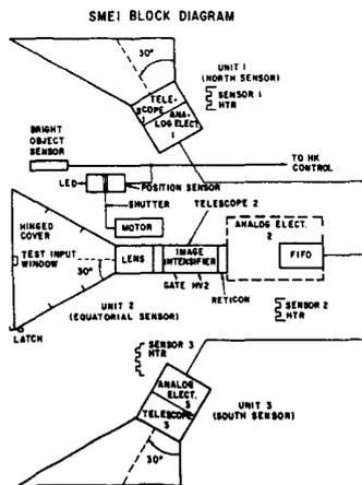
Fig. 2. Schematic of the proposed WIND spacecraft Solar Mass Ejection Imager front end; baffles, optics and electronics.
